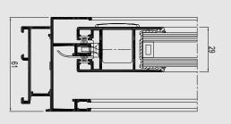
The CP 45Pa is a non-insulated sliding system that has been designed to respond to new aesthetical demands. The system is available in functional and softline design. The profile width is reduced to a minimum allowing a maximum of light into the building.
